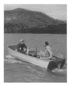
Tests showed the occupants of the boat, shown in the photograph, could talk in conversational tones, hear a portable radio or the lapping of waves over the engine while the motor was operating at its full throttle of five and a half horsepower.
