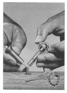
doors, replaces the inside push-down doorlock button on most cars. A pushbutton "snaps" the lock, shown in the photograph, but the ignition key is required to unlock it. The maker declares the device can be installed in one minute.
