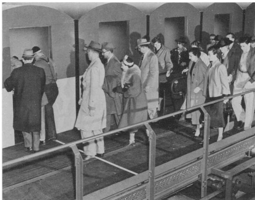
CONVEYOR-BELT TRAIN —Pretending they are harassed New Yorkers, these Aurora, Ill., citizens try out a prototype endless train of cars that runs on conveyor belts instead of rails. Such trains are said to hold many advantages over today's short shuttle subways.
