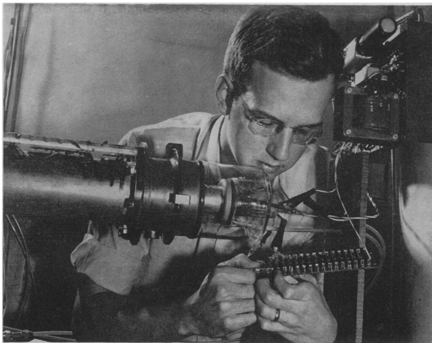
JUNIOR ANTI-CANCER ACCELERATOR —Six-million-volt electron "bullets" will be fired at cancer from this glass-enclosed "gun" being tested by Donald H. Janney, a graduate student at Stanford University. It is part of a junior-size linear accelerator being made for cancer therapy and industrial inspection.
