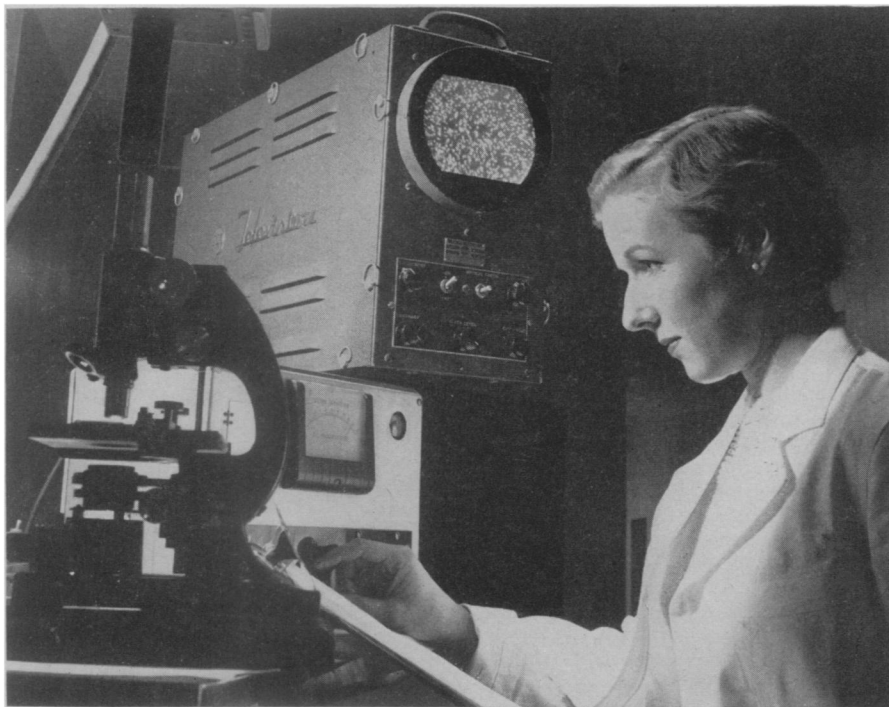
BLOOD COUNT BY TV —To make a quick count of human blood cells, an electronic "brain" has been joined with a television "eye" by scientists at RCA's David Sarnoff Research Center, Princeton, N. J.
