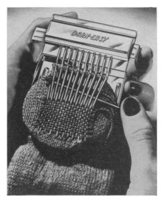
of the fabric to be mended are placed, as shown in the photograph. In a quick, single motion, the device turns the loops to eliminate "in-and-out" work. Especially designed for housewives and bachelors, the device is said to be 10 times as fast as hand work and gives more professional results.
