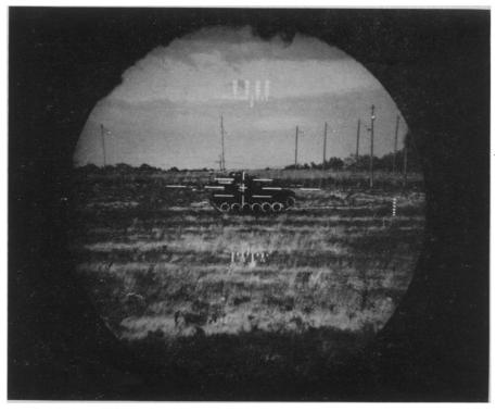
ON TARGET—Taken through the eyepiece of the Army's new range finder, this picture shows what a U.S. tank commander sees as he draws a head on his target, an M-47 medium tank. The new range finder automatically feeds precise distance of the target and proper ammunition setting into the tank's 90-mm gun as soon as the target is lined up.
