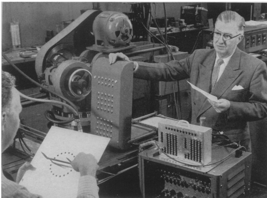
AUTOMATIC PUNCH PRESS —A forerunner to an automatic assembly machine, the work of the punch press is controlled by an electronic computer, which reads information on the size, number and location of holes to be punched from a perforated card. The techniques employed to make it automatic may also be applied to machines for drilling, riveting, etc., the General Electric engineers who developed the punch press state.
