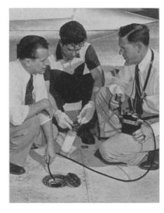
it emits enough carbon dioxide to nullify fire and explosion dangers. It was originally developed for use with the U. S. Air Force's F-89 Scorpion interceptor.
