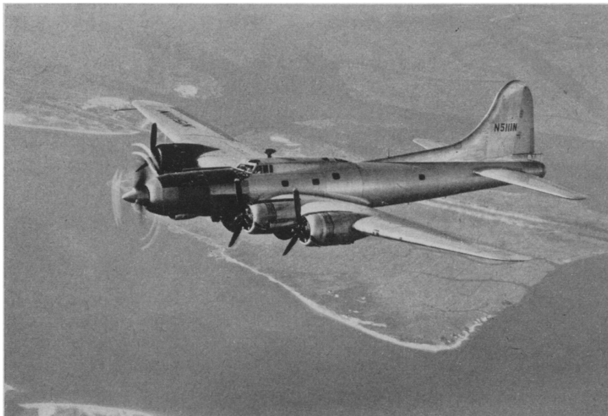
ENGINES FEATHERED —A single propeller-turbine powerplant, producing 5,700 horsepower, can propel a B-17 alone when its four piston engine propellers are feathered.
