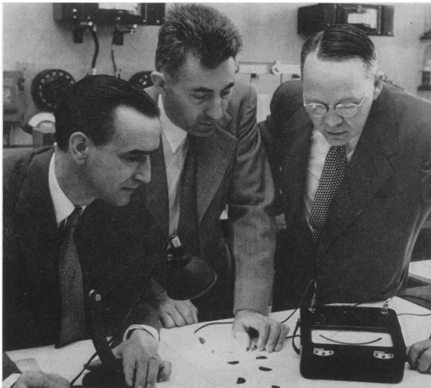
POWER CHECK-UP —Inventors of the Bell solar battery, G. L. Pearson, D. M. Chapin and C. S. Fuller, are shown checking sample devices for the amount of electricity derived from sunlight, here simulated by a lamp. The solar battery uses strips of silicon to convert the sun's energy directly and efficiently into electricity.
