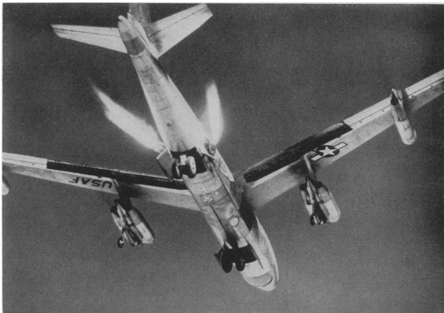
ROCKET'S ROAR —This Boeing B-47 is using the largest rocket power units ever designed for aircraft to become airborne. The liquid propellant rockets provide added power at take-off, permitting heavier payload and use of shorter runways. The power plants retract when not in use. Performance data have not been revealed.
