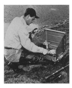
cylinders, as shown in the photograph. When not in use, the 16-pound stove folds into its own metal case.
