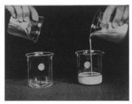
Now, in the beaker at the right is some lacquer made instead with a new low-viscosity cellulose acetate butyrate we call *Half-Second Butyrate* (from the length of time taken by a standard ball to fall through a standard length of a standard solution of the ester). Both it and its nitrate-based equivalent on the left were prepared 24 hours before the picture was made and treated alike.
