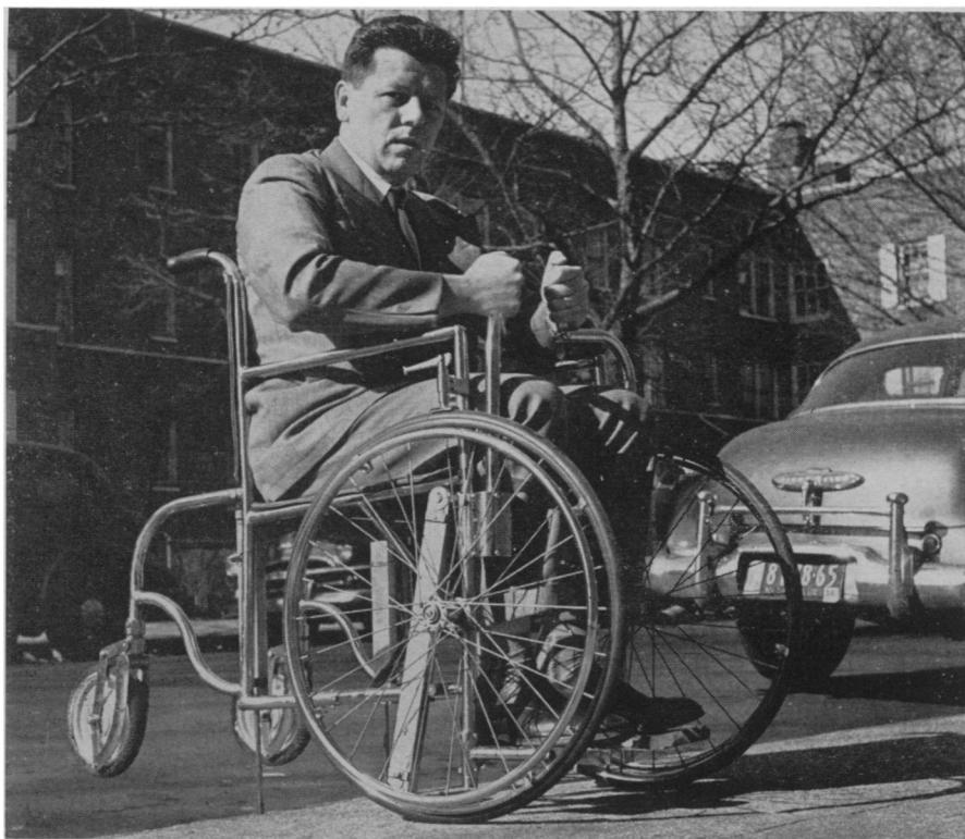
CURB-HOPPING WHEELCHAIR —With this new wheelchair, the invalid can get up and down curbs without requiring aid.
