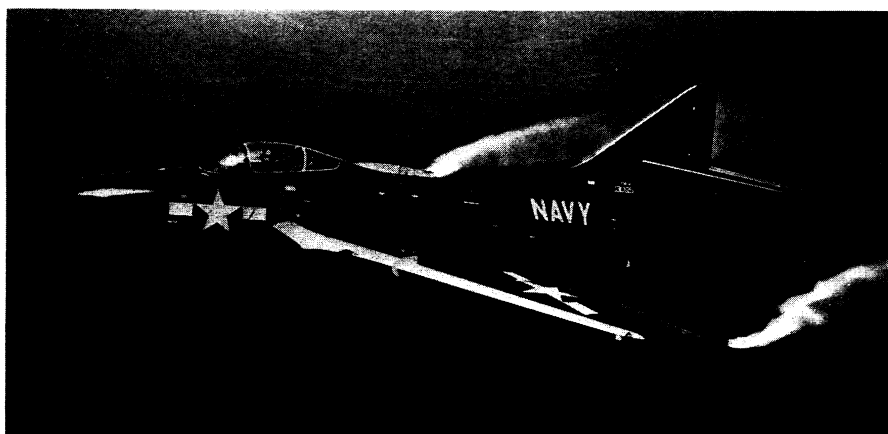
DUMPING FUEL FOR SAFETY —A Grumman F9F Cougar jet fighter releases the fuel from its wing tip tanks for safety reasons, a precaution taken just before landing to minimize danger of fire. Sparks from a dragging wing or similar mishap could send the expensive Navy fighter up in flames.
