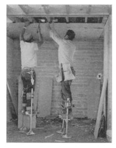
ADJUSTABLE STILTS for workmen and homeowners are made in 1¼-inch aluminum tubing and have 5x7½-inch nonslip bases, as shown in the photograph. They add up to 24 inches of height to the workman, obviating scaffolding and step-ladders
