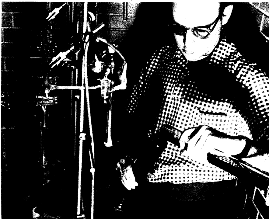
SOLUTION CERAMICS —New and flexible ceramic coatings can be applied to a wide variety of materials by the process of solution ceramics, developed at Illinois Institute of Technology's Armour Research Foundation. The coatings, whose liquid nature is shown in the photograph, can be sprayed at only a few hundred degrees Fahrenheit and will adhere to almost any solid surface.
