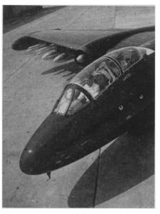
HIGH VISIBILITY—This close-up of the new B-57B shows the clear visibility provided for the pilot and also the second crewman who is seated behind him and slightly higher. It also shows half of the wallop packed in napalm tanks and high velocity rockets.
