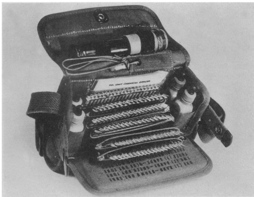
GAS DETECTOR KIT —Fast killing nerve gases and other war gases in the air have their presence shown by color reactions with the specially prepared silica gel in these clips.
