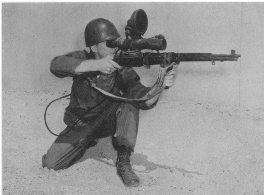
SNIPERSCOPE —This greatly improved version of the World War II model makes use of infrared light to permit a soldier to find his target in the dark without visible light. It is shown here mounted on an M-1 rifle. The improved version has a longer range, more rugged construction, and a more accurate aiming device than its older counterpart.
