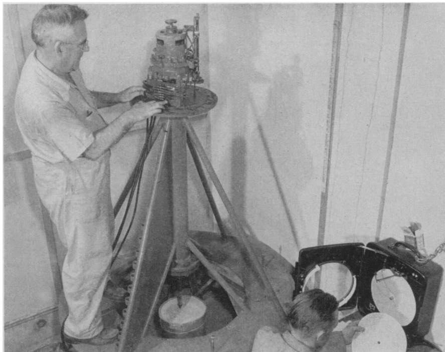
PENETROMETER —Dr. Clarence E. Miller, University of Rhode Island geologist is shown here adjusting an instrument he devised with Prof. John D. Nixon to measure the firmness of the sea bottom.
