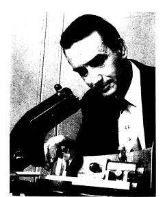
SOLAR BATTERY — A one-third increase in the efficiency of the Bell solar battery has been made. Here Gerald L. Pearson, a co-inventor of the battery, uses X-ray equipment to check the atomic structure of an ingot of silicon. The improved battery has an efficiency of eight per cent, comparable to that of steam and gasoline engines. (See SNL, May 1, p. 278.)
