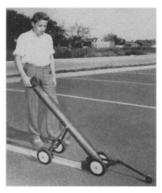
tional two-wheel assembly on the barrel that allows it to mark straight lines faster. Deliberate steering of the retractable guidewheel to right or left makes curved lines, and a slight lift of the handle raises the brush to allow skip lines.
