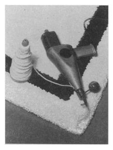
homemaker. This model is operated by a push-button trigger control and works at 90 strokes per minute. Weaving one-inch high, a loop rug can be done to the individual's own taste and pattern.
