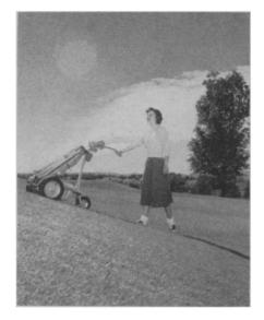
tograph. It features special gears to help pull the golfer up steep hills, as well as easing him down rugged grades. A handy handle switch stops and starts the device, and a speed selector paces the caddy to the individual's walking speed. Pneumatic tires and over-all light weight protect the turf.
