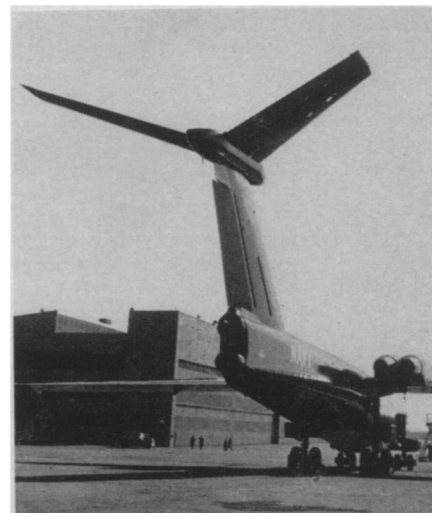
REAR VIEW —The "T"-shaped tail section of the Navy's new XP6M-1 SeaMaster towers three stories above the fuselage. The jet-powered, 600-mile-an-hour seaplane was designed for minelaying and photo reconnaissance.
