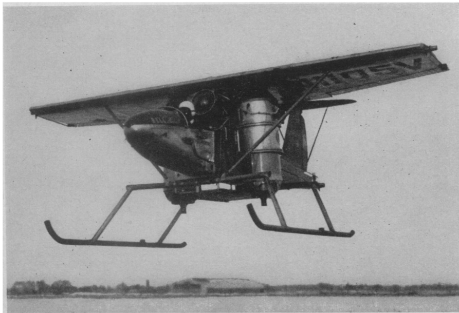
VERTICAL JET TAKE-OFF —Two turbojet engines with their thrusts directed downward raise this experimental airplane from the landing field. When the plane is airborne, the jets can be switched to horizontal position, and it can fly like a conventional plane. The revolutionary craft, developed by Bell Aircraft Corp., was successfully flown recently in tests.
