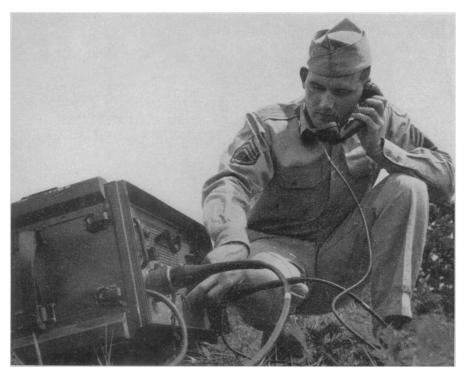
MILITARY PHONE—One of the new portable telephone systems that can handle four conversations at a time over a single cable is demonstrated in action. The repeater shown here is used to amplify the conversations, which may be transmitted over a distance of a hundred miles. Another, twelve-channel system, also developed by Bell Telephone Laboratories, can handle three times as many conversations over a single cable as comparable units used in World War II and Korea.
