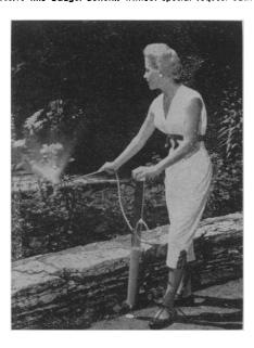
tom and is pushed down to operate sprayer. Up and down movement supplies pressure capable of shooting streams up to 10 feet from the ground. Sprayer head on a plastic wand has right angle turn to enable operator to spray all parts of plants or shrubs.
