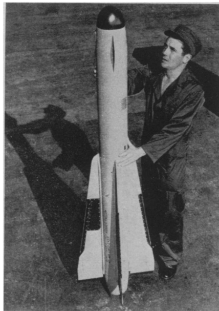
MISSILE WITH BRAIN — Size of the Falcon is compared to Air Force man. The deadly missile is six feet long and weighs 100 pounds.
