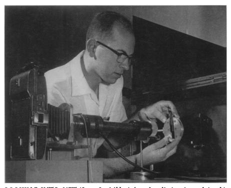
LOOKING INTO METAL — Invisible infrared radiation is used in this modified snooperscope to investigate the structural properties of silicon. Dr. William C. Dash, General Electric Research Laboratory physicist, places silicon in the light beam from an incandescent lamp, but of the total illumination only the infrared passes through, and is converted to visible light by the 'scope.
