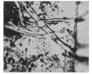
Here the plastic disc has picked up microscopic lint that insulates contact, stops current. (Picture enlarged 200 times.) Traces of contaminants are identified in microgram quantities. Inert plastic resists test chemicals that would damage contact.
