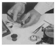
Preparing disc for microscopic examination. On-the-spot examination may reveal acid, alkali, sulfur, soot or other polluting agents peculiar to an area.
