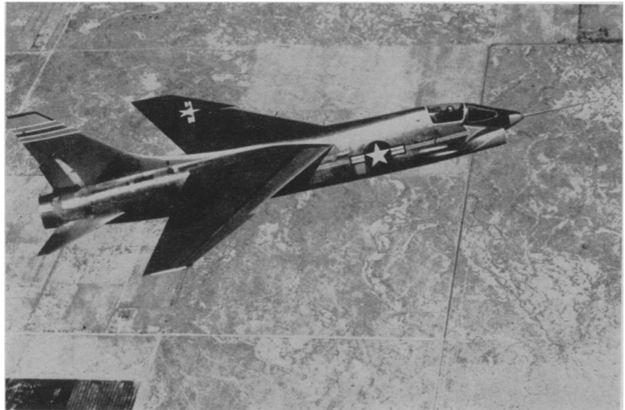
CARRIER-BASED FIGHTER —The Navy's supersonic jet fighter, XF8U-1, designed to operate from carriers, is now being tested. It can swiftly climb to more than ten miles, and is believed to fly about 900 miles an hour. Chance Vought test pilot John Konrad is flying the plane out of Edwards Air Force Base, Calif.
