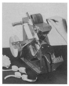
BOW TYER, shown in the photograph, turns out five gift-wrapping bows every two minutes, and can form hanks for over 100 bow variations. A turn of the gadget's handle forms a hank of ribbon that the operator puts through the notching mechanism and ties with a precut strip of narrower ribbon.
