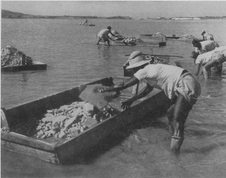
SALT FROM THE SEA —Natives of Araure, Venezuela, are shown gathering salt from flats that lie below the level of the sea. Sea water is constantly admitted through a system of canals to a depth of about two and one-half feet, at a rate determined by the evaporation. Salt in the water settles and crystallizes in layers that workers break with their feet, then toss by hand into barges.
