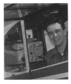
OR URANIUM DETECTOR, shown in the photograph, is designed for aerial prospecting from a small plane. The detector, a scintillation system, weighs less than 75 pounds, features low power consumption, and has an alarm that signals pilot and observer if any unusual radioactivity is detected.
