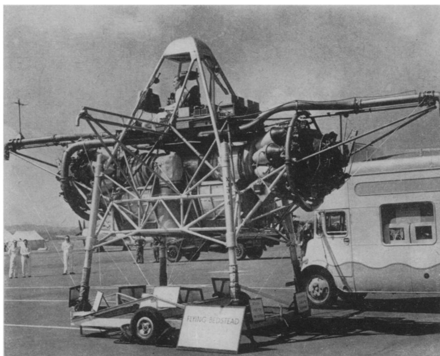
"FLYING BEDSTEAD"—Britain's experimental aircraft, built by Rolls Royce for studying the control of jets entirely by their jet thrust, can go straight up in the air from a horizontal position. The weird-looking plane was shown at the golden jubilee celebrations of the Royal Aircraft Establishment at Farnborough, Britain's main aircraft research center.
