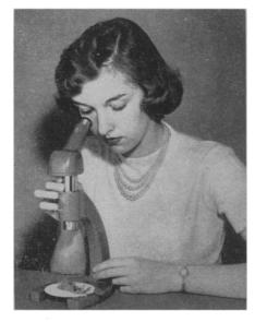
HOBBYIST'S MAGNIFIER, a microscope-like instrument designed for examining such things as stamps, coins, leaves and mineral specimens, provides an erect unreversed image of the object viewed. Field of vision is unusually wide and the only light needed is ordinary room illumination, as shown in the photograph.
