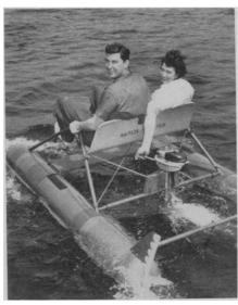
B PONTOON BOAT looks like a waterskimmer, those long-legged insects with a talent for skimming over the surface of still water. It is shown in the photograph. The boat's passengers are carried high above the water on a bench attached to two glass fiber pontoons. The boat is driven by passenger pedal-power, an outboard motor or an airplane-type engine.
