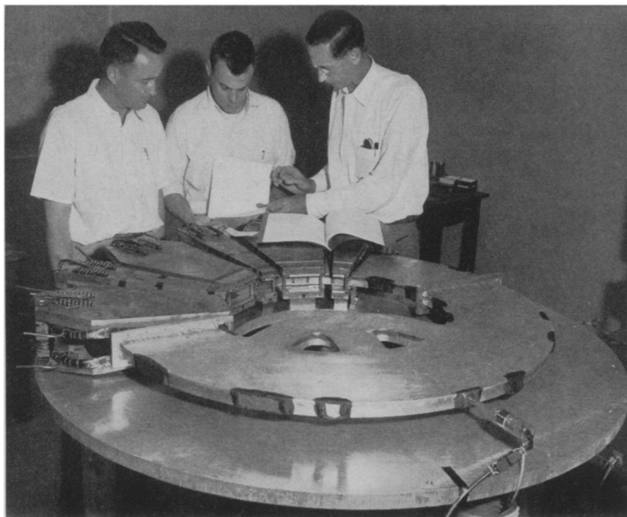
MODEL ATOM SMASHER —This one-ton model accelerator is being built at the University of Michigan to test a new principle for a 25-billion-electron-volt giant the Midwestern Universities Research Association hopes to construct in the Midwest. The design is expected to result in a simplified machine 100 times more efficient than existing atom smashers (see SNL, Feb. 5, p. 92). Pictured with the model are, from left to right, Drs. Kent M. Terwilliger and Lawrence W. Jones of the University of Michigan, and Dr. Donald W. Kerst, University of Illinois.
