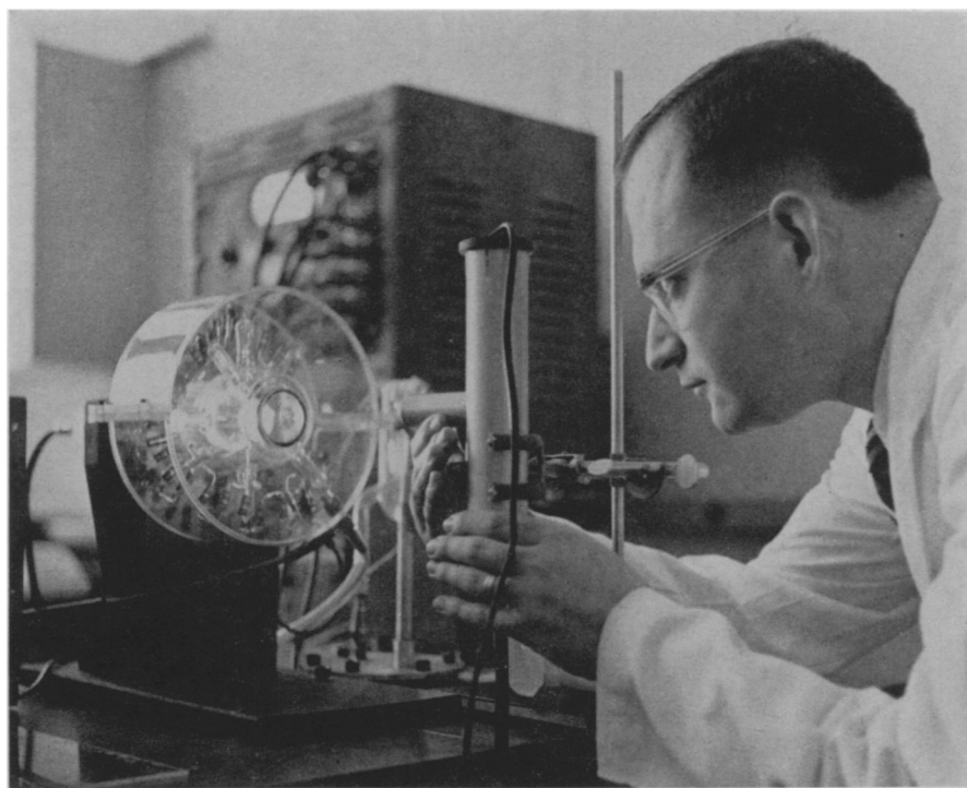
TIMING ATOMS IN FLIGHT —This electronic tube, capable of timing successive flashes of light less than one-billionth of a second apart, is the world's fastest "stop watch." It has an improved type of photomultiplier tube, using cascading electrons ejected from very thin films. Dr. E. J. Sternglass, research scientist at the Westinghouse Research Laboratories, Pittsburgh, Pa., adjusts a source of radiation beamed into the tube.
