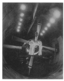
TURBOPROP PROP TEST— Checking a Britannia propeller made by de Havilland Propellers Ltd., workmen fit a pitch-change mechanism in the test tunnel at Hatfield, Hertfordshire, England.
