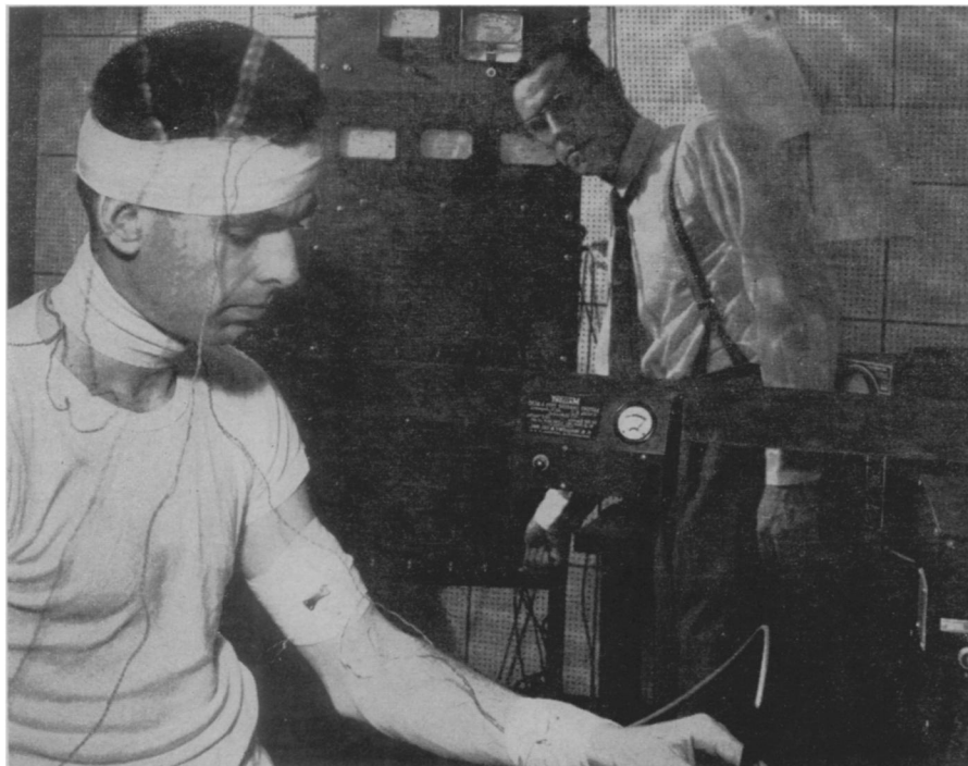
MEASURING MUSCLE POTENTIAL —Electronic techniques are being used to determine muscles' proficiency in work and play by Dr. Lee Gregg at Carnegie Institute of Technology, Pittsburgh, Pa. His electronic device measures muscle potentials, the tiny voltages generated in moving, in five body locations. The voltages represent muscle tensions, which indicate proficiency and strength of motivation. Dr. Gregg is shown in the background, separated from Brad Bunnell by a transparent steel-net shield.
