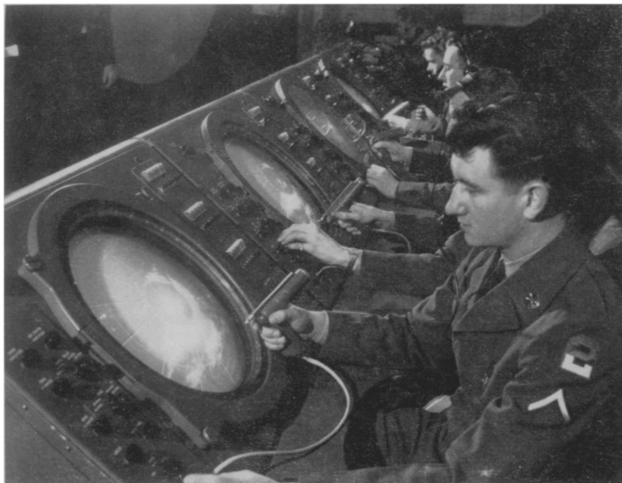
MISSILE MASTER —An electronic system to control and coordinate NIKE anti-aircraft missiles has been developed by the Army and Martin. Electronic consoles, similar to these radar entry consoles at Fort George G. Meade, Md., are the heart of the system. Here operators use photoelectric light guns placed against the screens to enter targets into the electronic tracking system.
