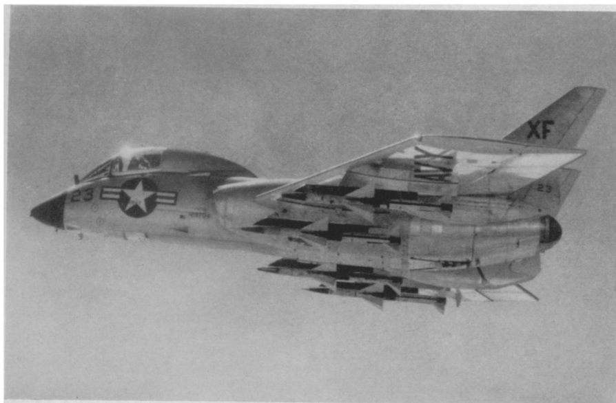
"SPARROW I" GUIDED MISSILE—Jet fighter planes of the U. S. Navy are now equipped with the air-to-air supersonic guided missiles known as "Sparrow I's." This photograph shows a Chance-Vought F7U-3M "Cutlass," after carrier launching, equipped with airborne guidance gear developed by the Bureau of Aeronautics and Sperry Gyroscope Company to direct the missiles singly or in groups.
