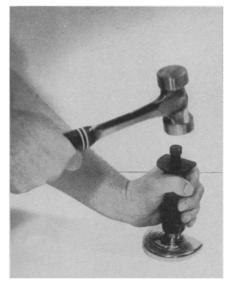
leveling plate is detachable so fastenings can be placed in corners. It comes in \% and \% inch sizes.
