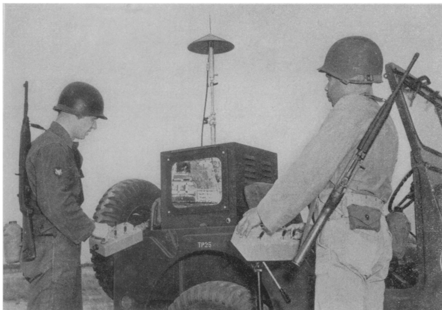
REMOTE TELEVISION —Soldiers shown here are operating by remote radio control a robot plane equipped with television. The unmanned aircraft sends back aerial pictures of sites up to 40 miles away, using light TV equipment developed at the Army's Signal Corps Engineering Laboratories, Fort Monmouth, N. J. Samuel Humes of New Paris, Pa., (left) operates the plane's ground remote-control box while William Howard of Baltimore Md., works the levers that point and focus the aerial camera.
