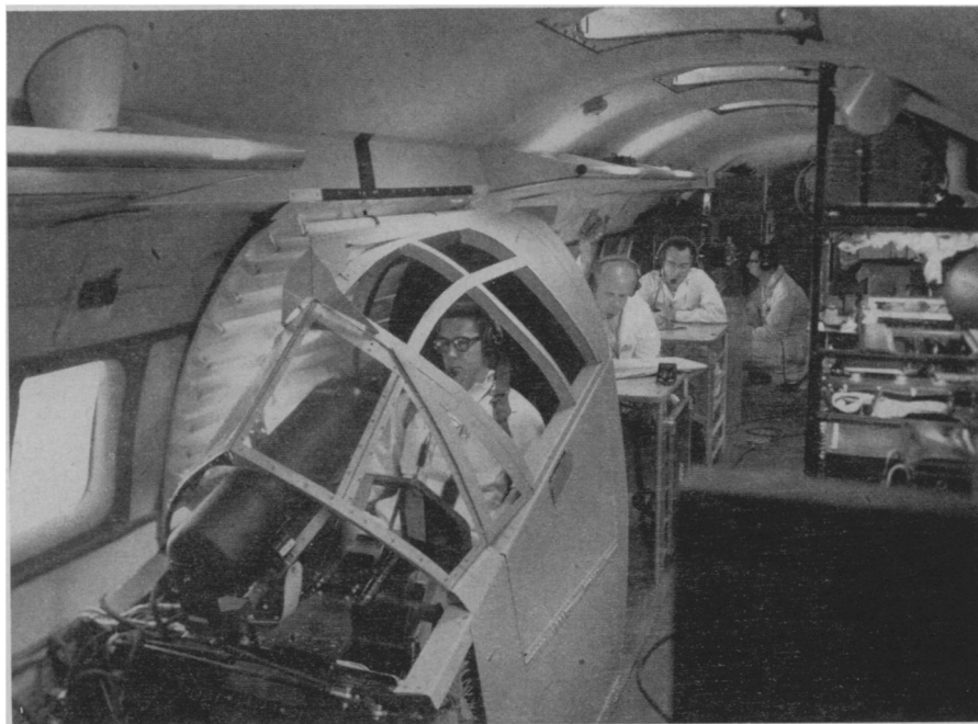
BACK SEAT FLYING —In a cockpit installed in the main cabin of a T-29 airliner, a second pilot takes over control of the airplane once the regular pilot has taken it aloft. Hughes Aircraft Company engineer R. E. Moore is shown in the "plane within a plane" where test pilots can fly as though they were in an F-102 jet interceptor while ten Hughes engineers can simultaneously check operation of the electronic control system.
