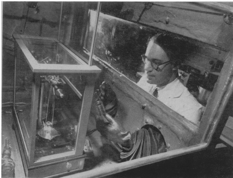
MAGNETIC MATERIAL — Scientists of the Westinghouse Electric Corporation have perfected a magnetic material, highly purified manganese-bismuth, that promises to yield powerful permanent magnets. Dr. Alex Goldman is shown here weighing a sample, which must be handled in the inert atmosphere of helium in order to avoid the spontaneous combustion that would otherwise occur.
